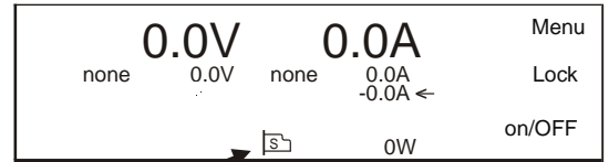
fig 3 -5 Position of the interface Slave icon in the unit display.
