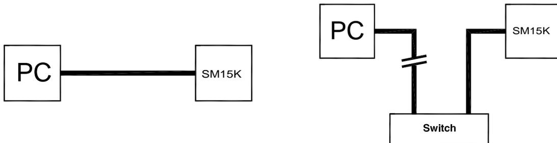
Either Cross-Link or standard Ethernet cable can be used. The command "PING <address>" of Windows® can be used (via menu Start - RUN - CMD) to check the connection. For example : PING 10.1.0.101
