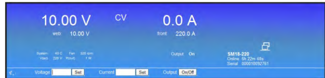
fig. 2 - 4, The front console of the web interface for setting of the input and monitoring various parameters.
