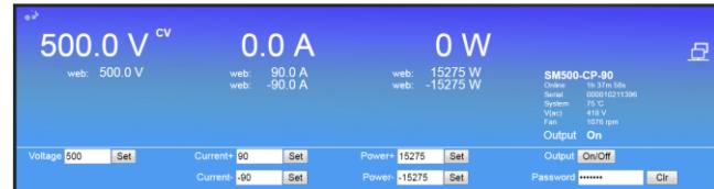
Figure 5.6: Remote display on web interface
