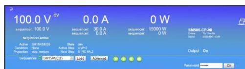
Figure 9.2: Sequencer console for selecting and controlling sequences.
