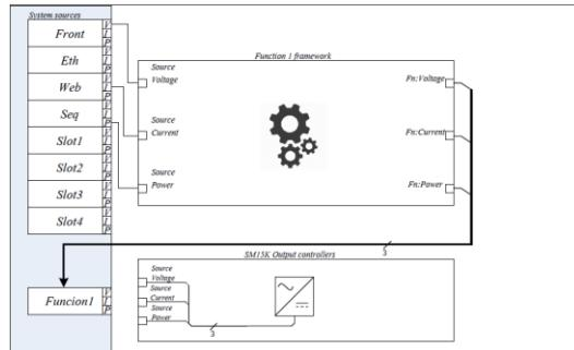
Figure 6.7: Functions Blocks can be put in between a program source and the units output controllers
