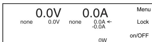
Figure 8.1: At the right side of the display, the 3 main menu items can be chosen.
