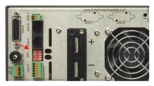
Set dip switch 5 of switch SW1 in the position 'down'. After switching mains on, the unit will always start up with a voltage setting of 0 V and a current setting of 0 A. Once the unit is switched on, the voltage and current can be set to the preferred value.
