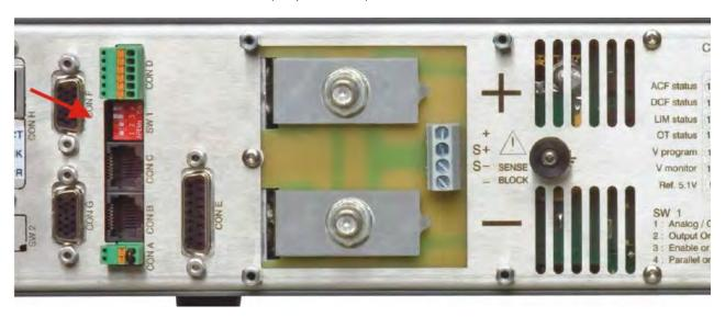
Set dip switch 5 of switch SW1 in the position 'down'. After switching mains on, the unit will always start up with a voltage setting of 0 V and a current setting of 0 A. Once the unit is switched on, the voltage and current can be set to the preferred value.
