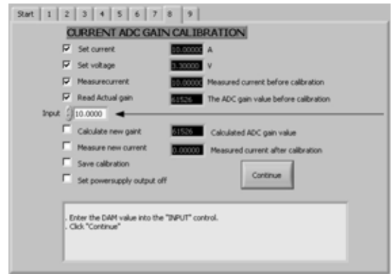
Screen 8: Current ADC gain calibration
