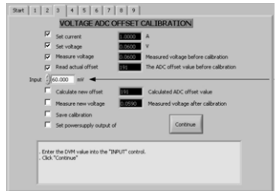
Screen 3: Voltage ADC offset calibration
