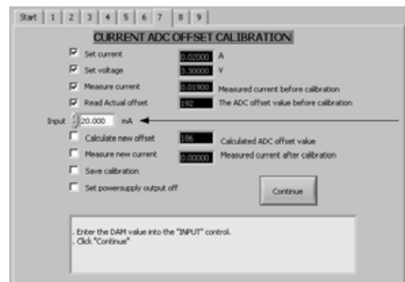
Screen 7: Current ADC offset calibration
