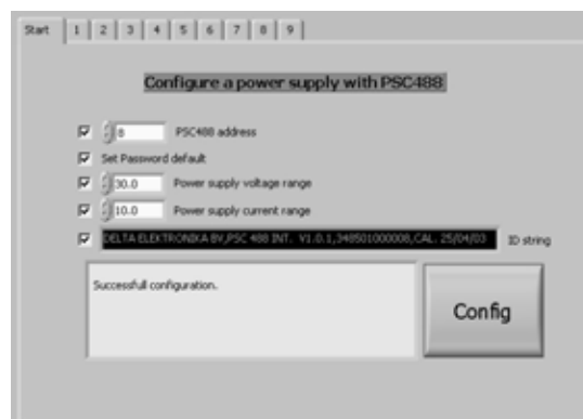
Start screen: Voltage and current configuration
