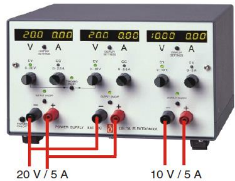
fig. 3 - 4 Parallel Tracking Mode
