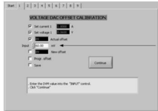
Screen 1: Voltage DAC Offset calibration
