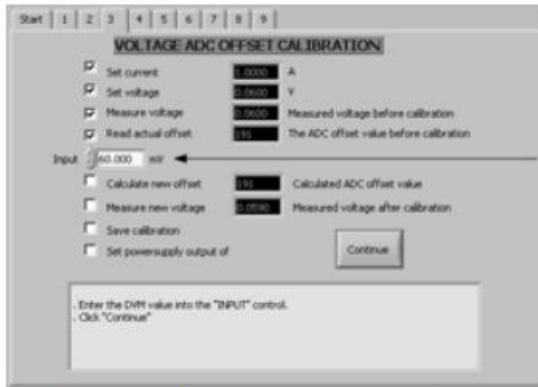
Screen 3: Voltage ADC offset calibration
