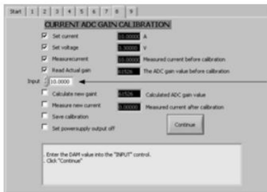
Screen 8: Current ADC gain calibration
