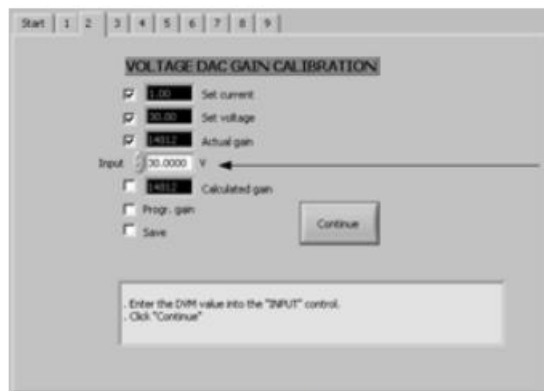
Screen 2: Voltage DAC gain calibration
