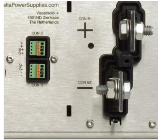
fig 6 - 3 The two DC power terminals CON B1 and B2. Con C and D are the sensing connectors.
