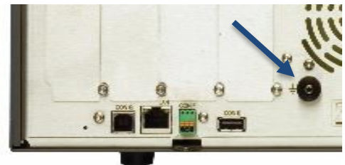
fig 4 - 4 Use this M4-size bolt for connecting at CBL2603.
