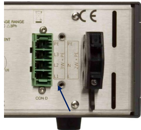
fig 6 - 1 Insert the included 4-pole header in CON D for the connection of the AC power / Mains.
