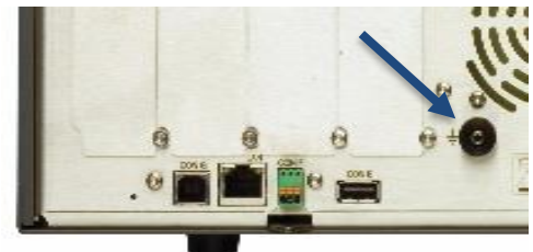
fig 4 - 4 Use this M4-size bolt for connecting al CBL2603.
