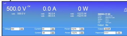
Figure 9.1: Front console for setting of the output and monitoring various parameters.
