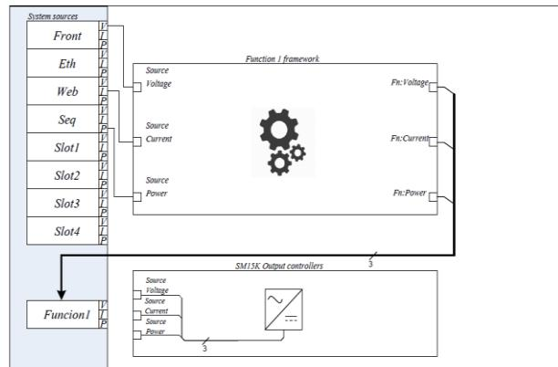
Figure 6.7: Functions Blocks can be put in between a program source and the units output controllers
