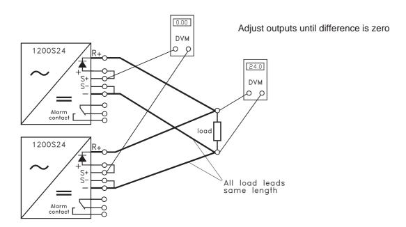
For redundant operation the 1200S units have a built in series diode and an undervoltage alarm contact. This contact can be used as normally open or as normally closed.
