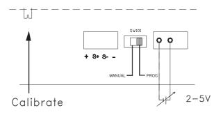
Attention: The programming input is not isolated. The zero of the progr. input is connected to minus output. When the small switch near the programming input is put on PROG (program) the output voltage of the power supply can be programmed by an analog voltage of 2 to 5V, corresponding with 12 to 30 V out-
