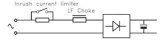
The inrush current limiter limits the inrush current to less than 40 A during 5 milliseconds. At turn on the electrolytic capacitors charge through a PTC series resistor of about 40 Ohms. When they are charged sufficiently the series resistor is shorted by a heavy relay contact and the power supply starts operating. In case of a relay failure the PTC becomes high ohmic and limits the current to a safe value.
