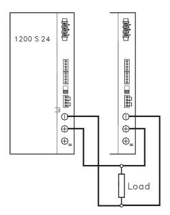
To obtain higher current two or more units can be used in parallel. Before connecting them in parallel first adjust each output to the same voltage. The current limit switch of the 1200S models has to be put on 'LO' to limit the
