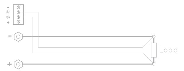
For most applications remote sensing is not necessary. However, if the voltage at the load has to be kept very constant (within millivolts) and the voltage drop across the load leads is large, remote sensing is useful. With remote sensing the voltage is kept constant across the load instead of at the output terminals of the power supply.
