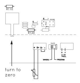
Voltage adjustment with an external potentiometer of 10 kOhms is possible if R 120 and R 110 are removed. The potentiometer can be connected as a variable resistor between S+ and + at the sense block. The internal potmeter has to be turned to zero.
