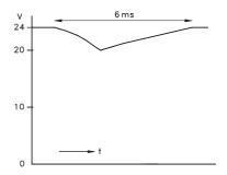
In the above situation there is still a considerable voltage dip during 6 ms. This can be improved by one or more large electrolytic capacitors which can supply a high current peak for a fast action of a fuse or a circuit breaker.
