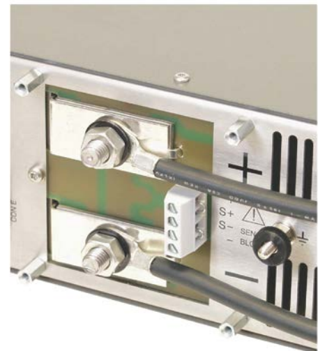
fig 5 - 1 Low resistive cable connection by mounting the cables directly on the DC output strips.
