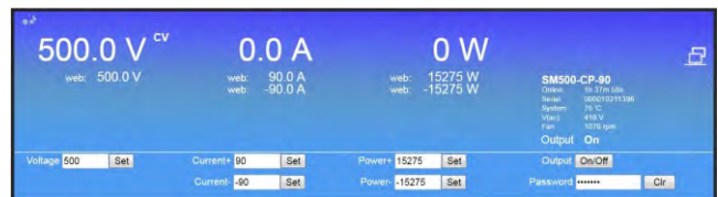
fig. 2 - 4 The front console of the web interface for setting of the output and monitoring various parameters.
